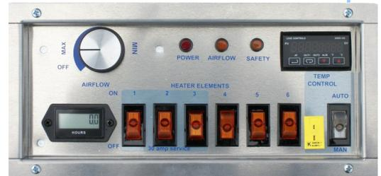
**Heating Elements**....6 - Tubular, finned elements, 11kW; Temperature rise is 75°F at 475 CFM airflow (95°F at 350 CFM)
