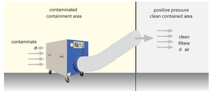
To create **POSITIVE PRESSURE** inside the containment, more air has to be pumped in than leaks out of the containment. Place the machine outside the containment and hook a flexible duct to the inlet ring of the machine ducting the exhaust into the containment. (See Above)
