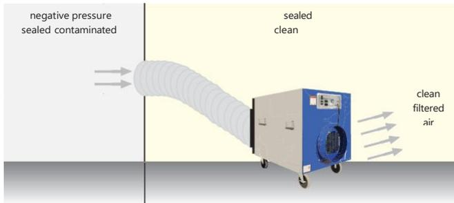
To create **NEGATIVE PRESSURE** inside the containment, more air has to be exhausted out than leaks into the containment. Place the machine inside the containment and hook a flexible duct to the outlet ring of the machine exhausting to outside the containment.
